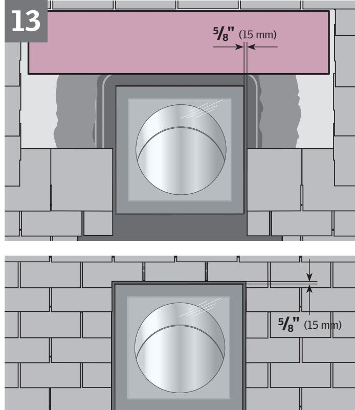
**ENGLISH:** Reinstall roofing material over the flange. Leave a  $5/8"$  (15 mm) channel for water to run off.
