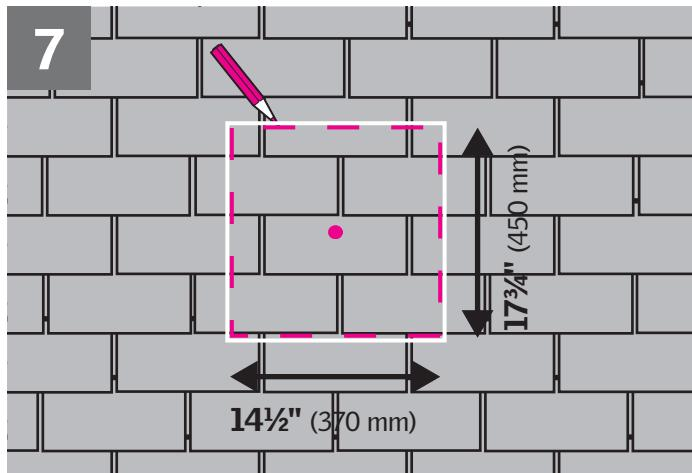
**ENGLISH:** Locate the nail indicating the center of the sun tunnel on the roof and mark rough opening.
