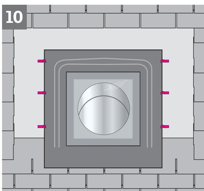
**ENGLISH:** Center the flashing over the rough opening and secure the flange with clips and nails provided.
