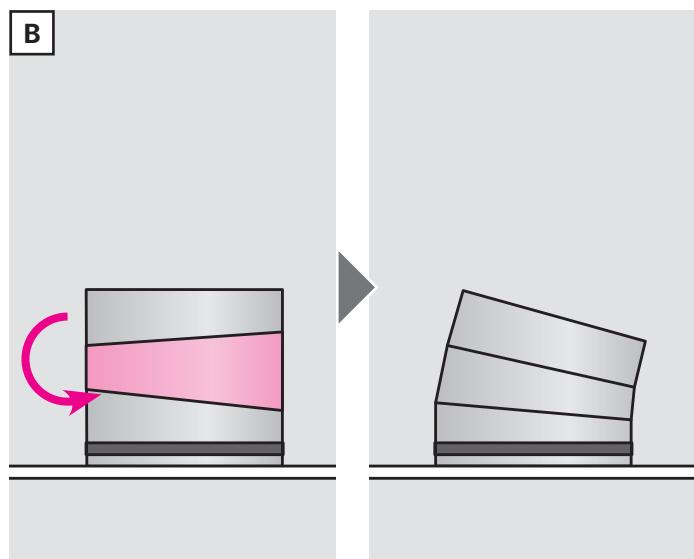
**ENGLISH:** Adjust the angle of both elbows so that they point directly against each other **A**, **B**. Elbows can be damaged if excess force is applied.
