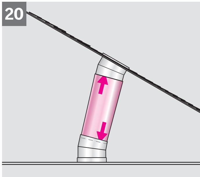
**ENGLISH:** If necessary, cut the rigid tunnel section to length **A**. Reduce the length of the tunnel section by increasing overlaps. Secure all joints with two of the  $\frac{3}{8}$ " (10 mm) screws **B**.
