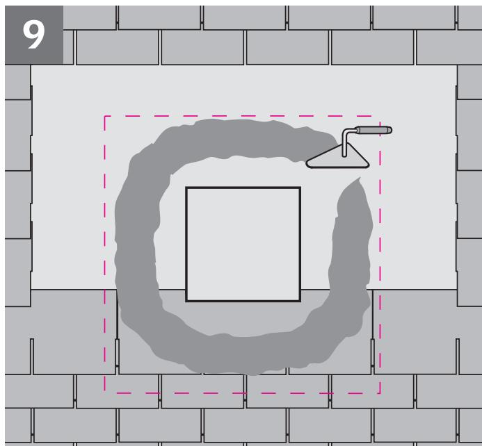
**ENGLISH:** Remove the roofing material around the upper half of the rough opening as indicated and apply mastic around rough opening as shown.
