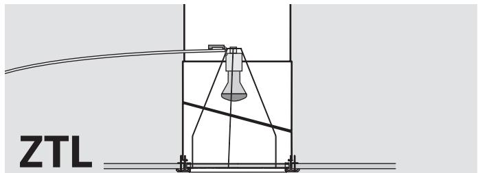
**ENGLISH:** If vapor barrier is installed, insure a tight joint between the ceiling ring and the vapor barrier. Reposition the insulation material around the tunnel.
