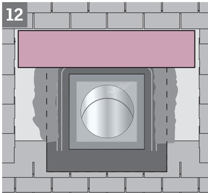
**ENGLISH:** Overlap the top of the flange with underlayment to allow for proper drainage.
