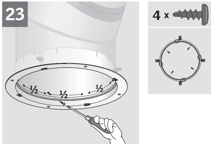
**ENGLISH:** Secure tunnel assembly to ceiling ring with four of the  $\frac{3}{8}$ " (10 mm) screws provided.
