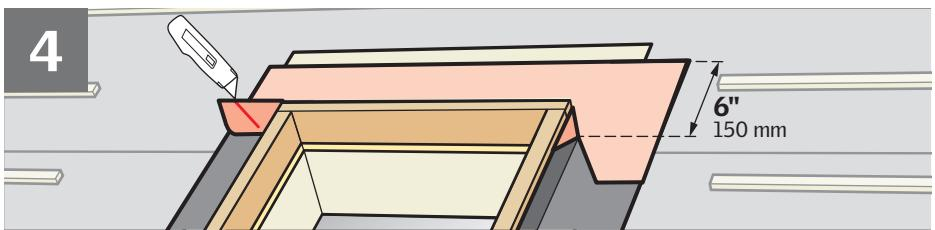
**ENGLISH:** Wrap the top and the corners of the skylight curb with VELUX adhesive skylight underlayment and create proper water-shedding lap.
