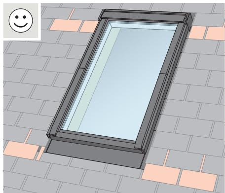
**ENGLISH:** Observe distance to roofing material. Do not nail through the saddle flashing when attaching the roofing material.
